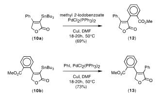
In summary, we have demonstrated that the regioselective Stille reaction of bis(stannane) **3** allows preparation of 4-substituted 3-stannyl-2(5*H*)furanones **10**; current research is directed toward optimizing the yields of the process and extrapolating the range of coupling reactions thus far examined.
